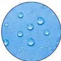
Fluid-repellent SMS material
